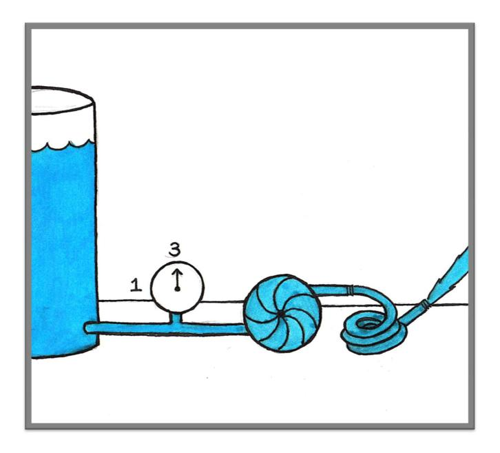
PRS-04: The second article of equipment necessary for pressure rinsing takes the *form of a static* or rotating spray jet of water. The jets of water hit the internal surfaces of the container removing and dissolving the pesticides residue.
