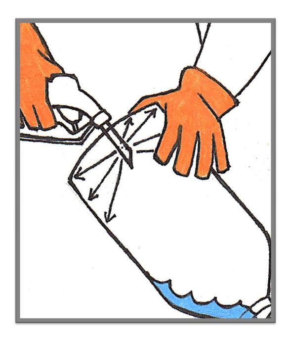
PRS-05: Some pressure rinsing equipment includes a sharp device that penetrates the container walls for rinsing purposes, thereby offering the additional advantage of making the container unusable...
