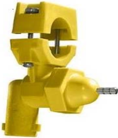
CP-112SE— \frac{1}{2} " split eyelet CP-112SE1—1" split eyelet Quick coupler outlet 5.2 GPM at 40 PSI 30% Glass filled yellow nylon
