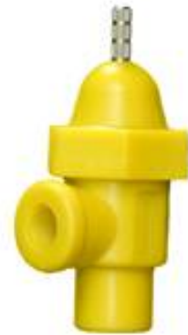
CP-04— \frac{1}{8} " Female Inlet \frac{1}{8} " Female Outlet 5.2 GPM at 40 PSI 30% Glass filled yellow polypropylene
