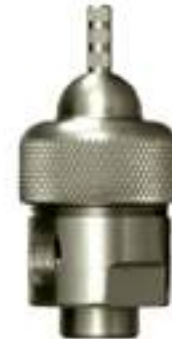
CP-02— \frac{1}{8} " Female Inlet \frac{1}{8} " Female Outlet 5.2 GPM at 40 PSI Stainless Steel
