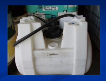
Question 5: This is a new tank that the registrant says meets the DOT standards, but it does not have the UN marking on it. Would this container meet EPA's requirements?
