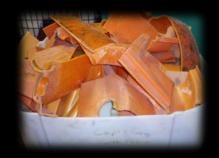
Step 1- Tanks are stripped of metal, and prepped into 18" or less squares
