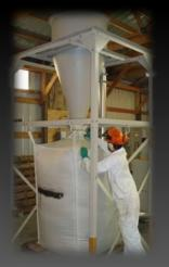
Step 3 – granules are air conveyed into bulk Bags and prepared for transportation
