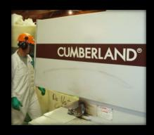
Step 4- Granules are brought down to 3/16" grind and run through a wash line in preparation for end use marketing
