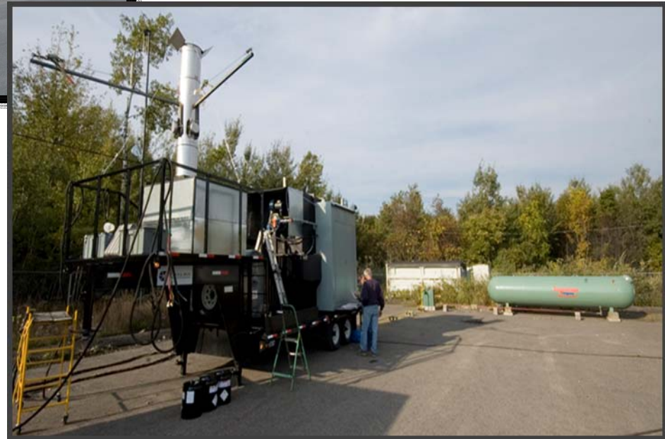
FRALMA Unit during tests showing sample probes on Chimney
