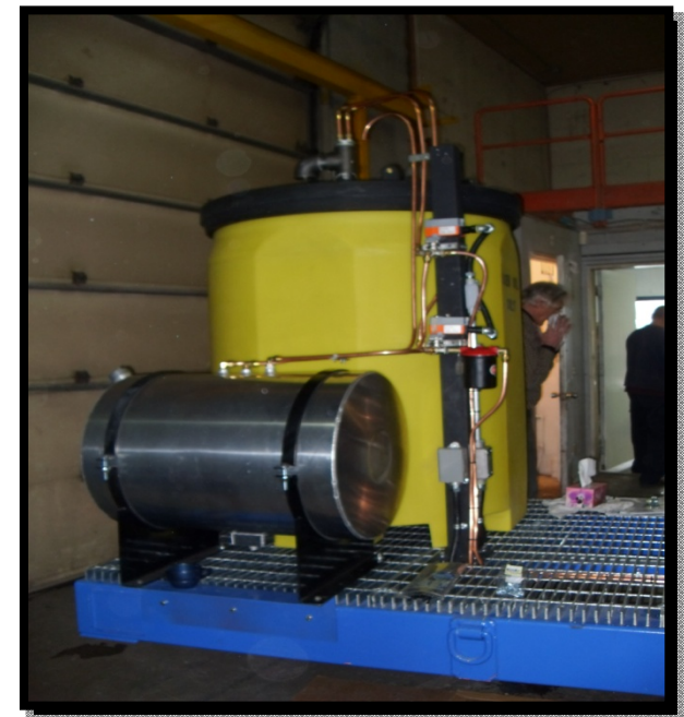
PCBs contaminated oil or pesticides tank
