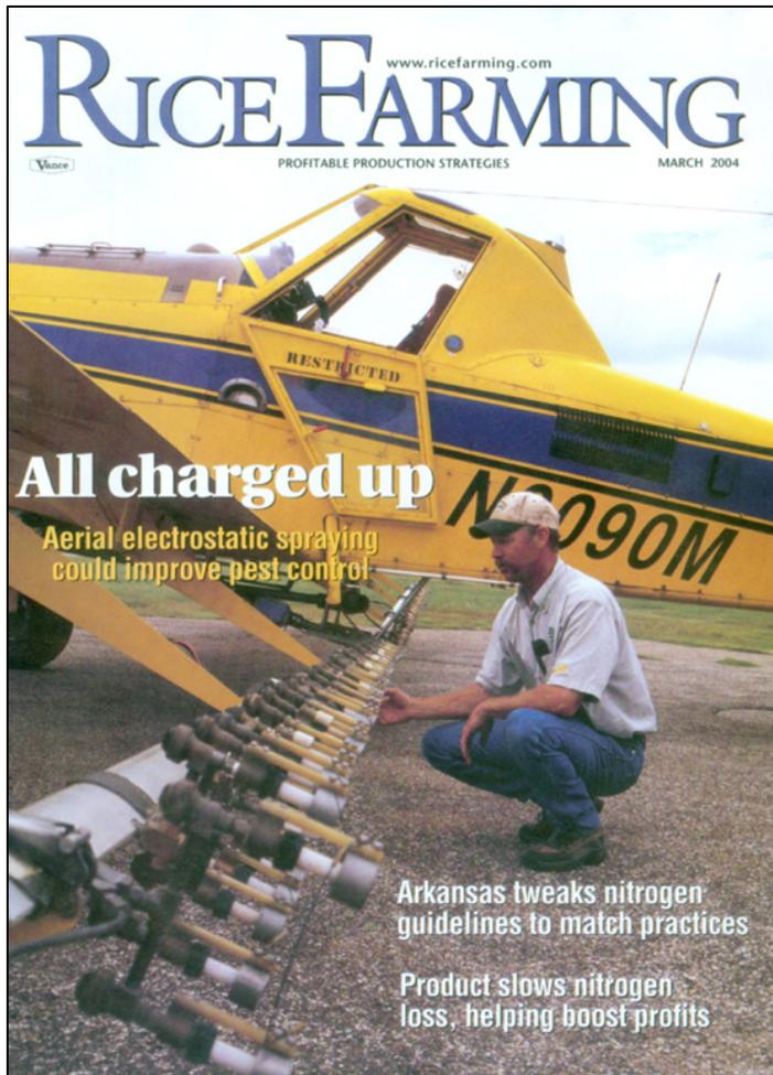
**Electrostatic Nozzles—** developed by ARS—induces the chemical droplets with either a positive or negative charge before their release over the target. Charged aerial sprays are attracted to targeted objects such as crops, trees and other plants. Electrostatic nozzles can be very beneficial in the aerial application industry because you can use less carrier per acre with the active ingredient; hence you can apply more acres per load. This means less fuel used.
