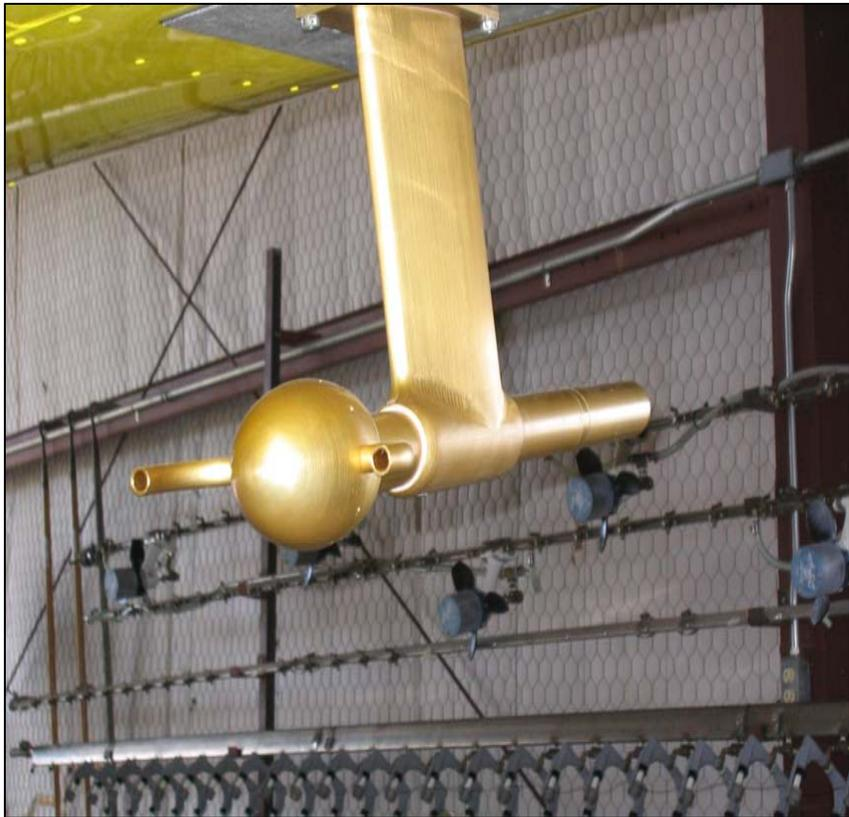
**Aircraft - Integrated Meteorological Measurement System (AIMMS) measures site specific atmospheric turbulence data to support aerial application, including wind speed, direction, altitude, humidity and temperature.**
